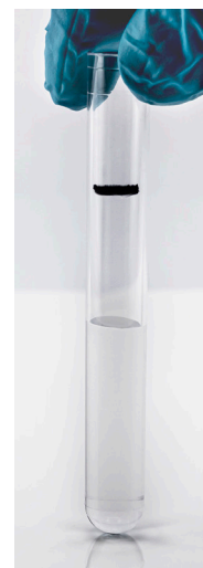
Figure 1. Shows the remaining 3.5 mL of sample post analysis – the black line indicates the original level of the 6 mL extract. Samples can be reanalyzed without re-extraction.
